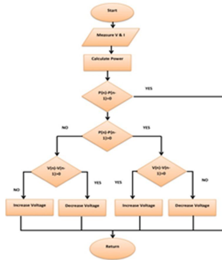
Fig. 3 Flowchart of Perturb & Observe algorithm
